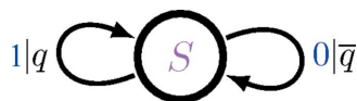
Figure 3 Hagg-machine for the IID process. When q = 1 , the IID process generates a string of 1's, which is physically the 3C^+ stacking structure. Conversely, when q = 0 , the structure corresponds to the 3C^- structure. For q = 1/2 , the MLs are stacked as randomly as possible. Here and elsewhere we adopt the convention that a bar over a variable means one minus that variable, i.e. \bar{q} \equiv 1 - q , with q \in [0, 1] .
